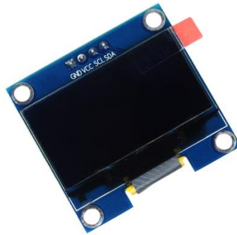
0.96 Inch 128X64 Blue OLED Display
